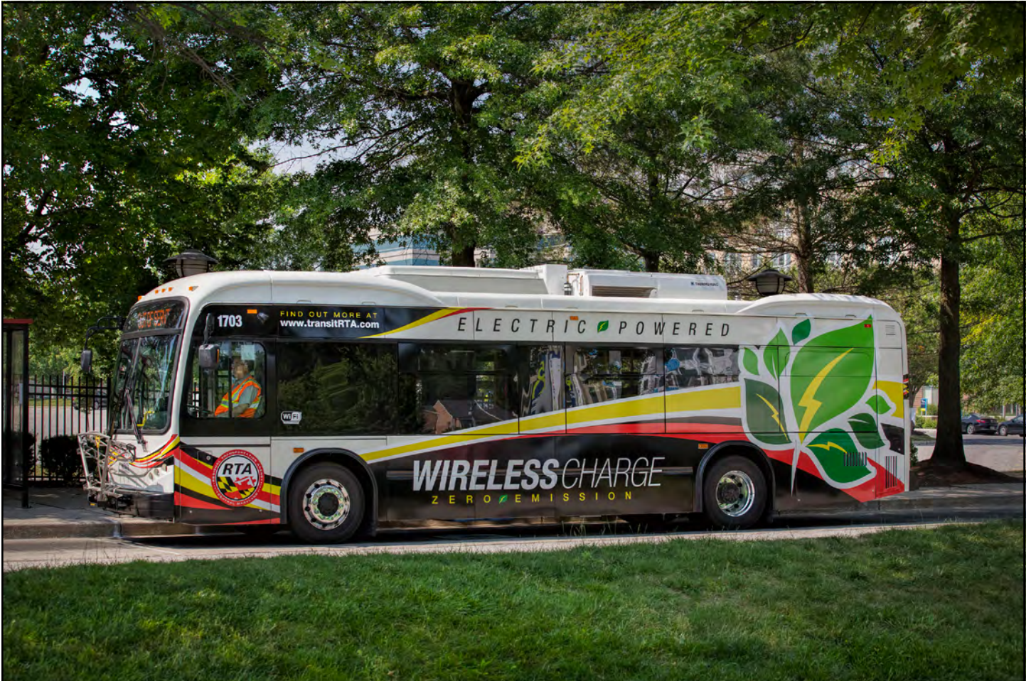
Electric buses operating RTA Route 401 recharge wirelessly at the Mall in Columbia.
